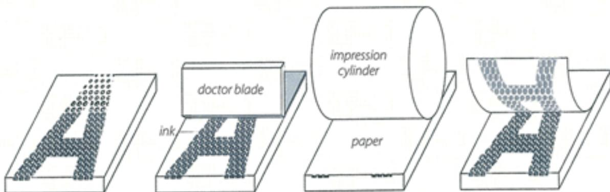
A diamond stylus or chemicals engrave the wells. A scanner reading a halftone positive guides the stylus.
